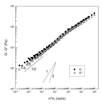
Fig. 8. Dynamic oscillatory shear data in the form of G' and G'' master curves for tri-block copolymer  $p(MA-POSS)_{10}$ - $b-p(BA)_{201}$ - $b-p(MA-POSS)_{10}$ . The reference temperature for time-temperature superposition shifting was  $T=80\,^{\circ}\text{C}$ .
