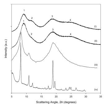
Fig. 7. Powder patterns of wide-angle X-ray scattering (WAXS) using Cu K $\alpha$  radiation ( $\lambda=1.5418$  Å) for (i) p(MA-POSS) homopolymer following annealing at T=55 °C for seven days (same as DSC trace c (i) for Fig. 5); (ii) p(MA-POSS) homopolymer as isolated after fractionation; (iii) POSS triblock copolymer, p(MA-POSS)<sub>6</sub>-b-pBA<sub>481</sub>-b-p(MA-POSS)<sub>6</sub>; and (iv) MA-POSS (cyclopentyl) monomer.
