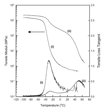
Fig. 3. Dynamic Mechanical Analysis (DMA) comparing POSS-triblocks of varying poly(butyl acrylate) central block molecular weight: (i) p(MA-POSS) $_6$ -b-pBA $_{481}$ -b-p(MA-POSS) $_6$  and (ii) p(MA-POSS) $_{10}$ -b-pBA $_{201}$ -b-p(POSS-MA) $_{10}$ . Tensile films were prepared be solvent casting and temperature sweeps conducted at a heating rate of 4 °C/min while applying oscillatory strain of approximate magnitude 0.1% and with a frequency of 1 Hz.
